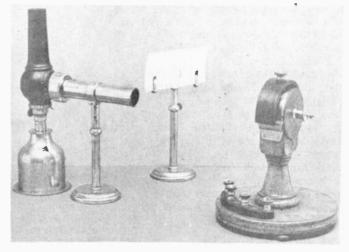
Fig.5. Kelvin's mirror galvonometer (1858). The oil lamp, at left, provided a light beam that was deflected by a mirror mounted on the coil of the galvanometer at right. The deflected beam moved across the calibrated scale at centre.
