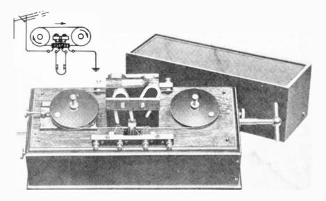
Fig.7, Marconi's magnetic detector of 1902,
