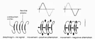
Left: The Heil driver unit as seen from above. Above: Electrical audio signals cause the accordian-like pleats to open or close (depending on the polarity of the signal).
