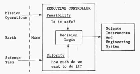
Typical control system. On-board executive controller monitors data relating to robot's environment, ie, internel and externel temperatures, power evailability, wind speed, terrein, instrumentation condition atc, it then compares this against stored data relating to mission priority and desirability and then decides whether or not mission should proceed. The robot's decisions can at any time be overridden or modified by earthbased mission operating centre.
