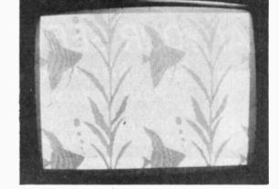
Fig. 7. The designer needs only to produce one cycle of the pattern — the computer-based colour display repeats it to provide a view of the complete pattern.
