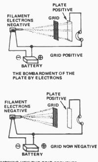
SHOWING HOW THE GRID PREVENTS THE ELECTRONS FROM REACHING THE PLATE
