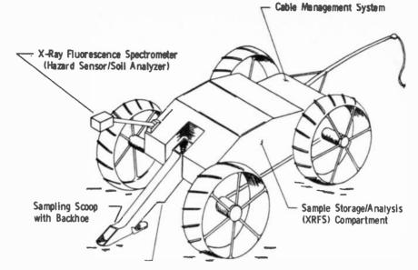
Fig.2. Tethered rover associated with advanced lander.
