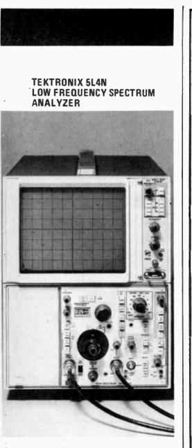
The new 5L4N is a 0-to-100 kHz spectrum analyzer that offers both high performance and economy. Tektronix state that the analyzer has unique features including push-button selection of 50 ohm, 600 ohm or 1 input impedance megohm with calibration appropriate to the selected impedance.
