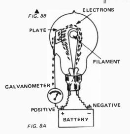
filament (cathode) and the plate (anode) if the grid is left unconnected. Signals connected to the grid either allow or prevent this action depending upon their polarity and magnitude – as shown in Fig. 9. A small varying signal voltage applied to the grid controls the flow of a large current in the anode circuit, thus obtaining gain (by producing a signal larger than that fed in).
