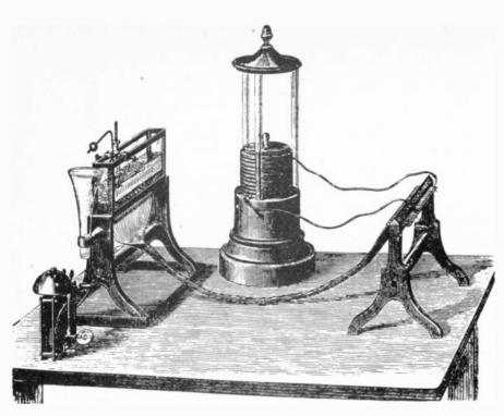
Fig.3. Sommering's 1810 electrolytic detection telegraph. The central voltaic pile provided electric current that was applied to the channel representing the letter to be sent. Current at the receiving end (LHS) produced gas, by electrolytic action; which raised the balanced spoon and caused a lead ball to drop through the funnel onto the bell. It really worked but the problem of finding which channel was in use must have been time consuming.
