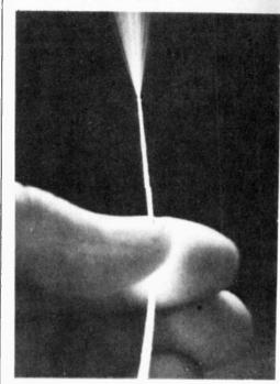
Like water from a hose, light pours out of the end of this nearly one kilometre length of light fibre.
