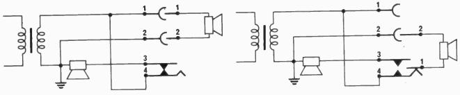
Fig. 1a. Example of using the type 05 connector inserted in position A, Both speakers are operational.
